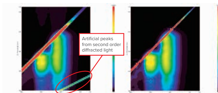
3D Spectra of Fluorescent Orange Color Plate Left: Without Cut-Off Filter Right: With Cut-Off Filter
