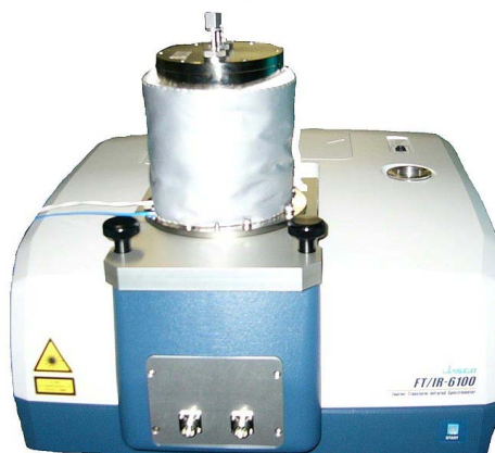
Figure 1. Full vacuum type FT-IR gas analysis system (10 meter cell)
