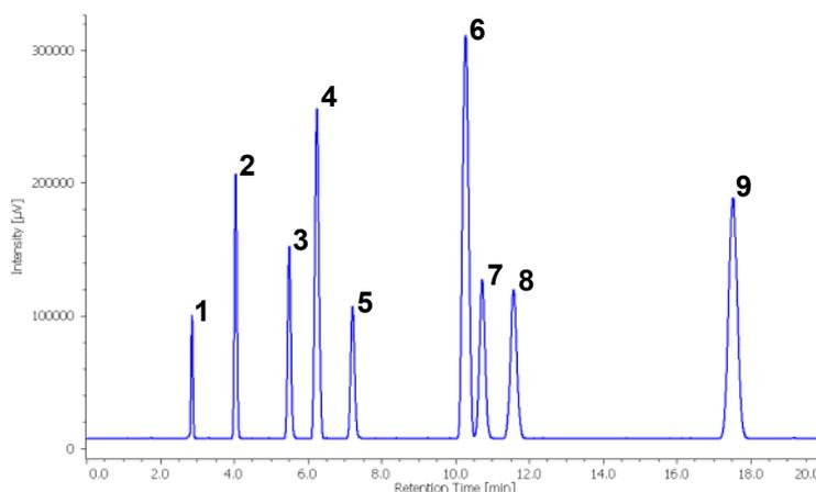
**Fig. 1.** Chromatogram of standard mixture of 9 fatty acids including trans fatty acids
