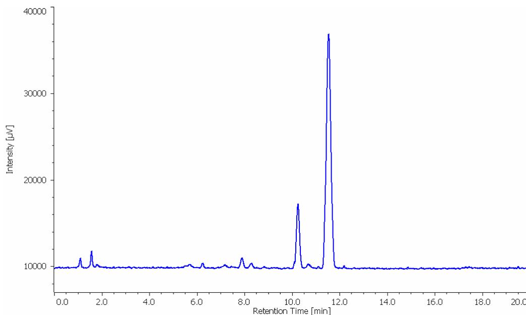
**Fig. 5.** Chromatogram of Margarine added with Elaidic acid
