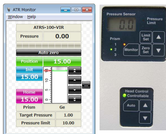
Fig. 2. Pressure monitor (left) and operation panel (right)
